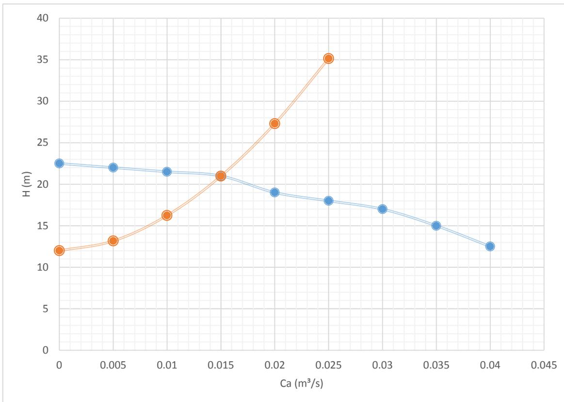
When I reviewed my chart, I found out that the point of intersection of the two curves, or the pump operation point, had a head of 21 m and a flow rate of 0.015 m<sup>3</sup>/s.
