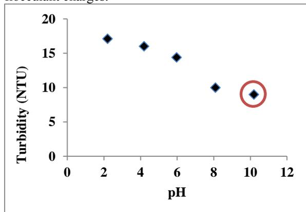
**Figure 2: Evolution of turbidity as a function pH solution (V=500mL, Dose= 1mL of the flocculant, time=60min)**
