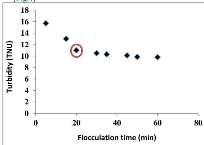
**Figure 4: Effect of flocculation time on Kaolin flocculation (pH=10, V=500mL, Dose=1.5mL of the flocculant).**
