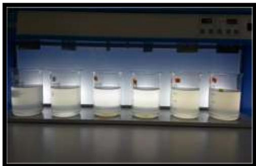
**Figure 1: Jar test system for suspension matter elimination**
