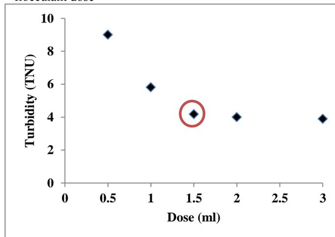
**Figure 3: Effect of the flocculant dose Kaolin flocculation (pH=10, V=500mL, time=60min)**
