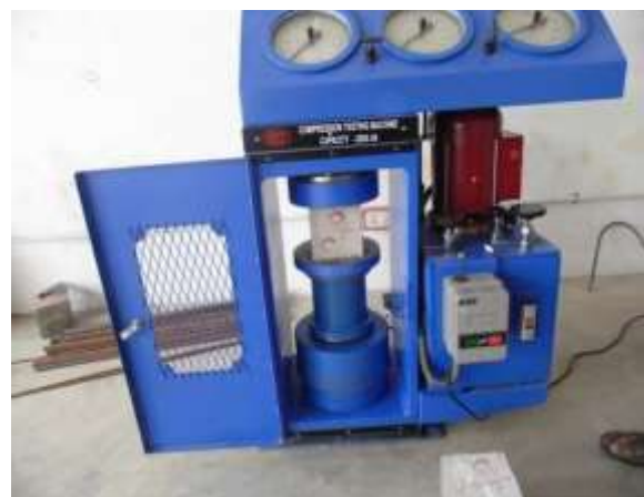
Fig. 3 Compressive testing machine Tensile strength test procedure
