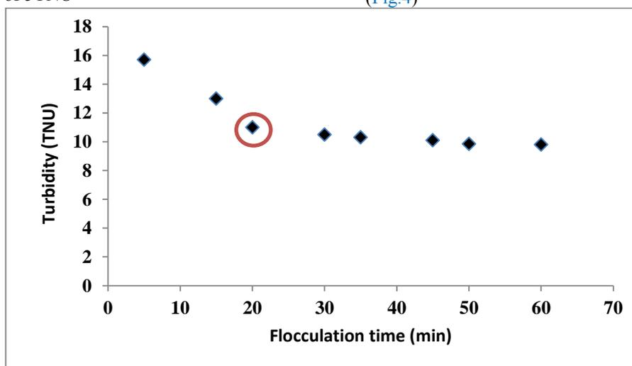
**Figure 4: Effect of flocculation time on Kaolin flocculation (pH=10, V=500mL, Dose=1.5mL of the flocculent).**
