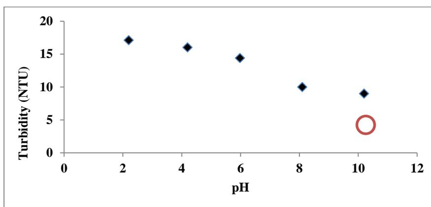
**Figure 2: Evolution of turbidity as a function pH solution (V=500mL, Dose= 1mL of the flocculant, time=60min)**
