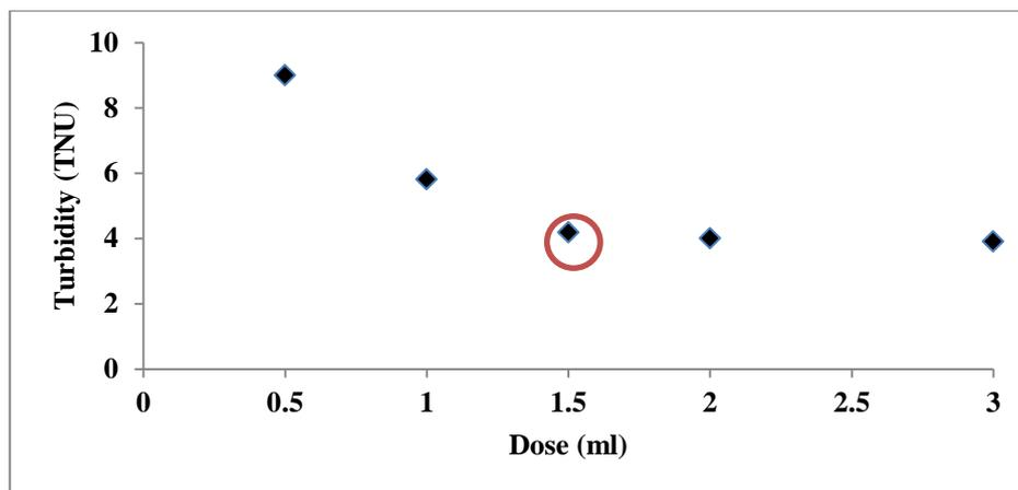
**Figure 3: Effect of the flocculant dose Kaolin flocculation (pH=10, V=500mL, time=60min)**
