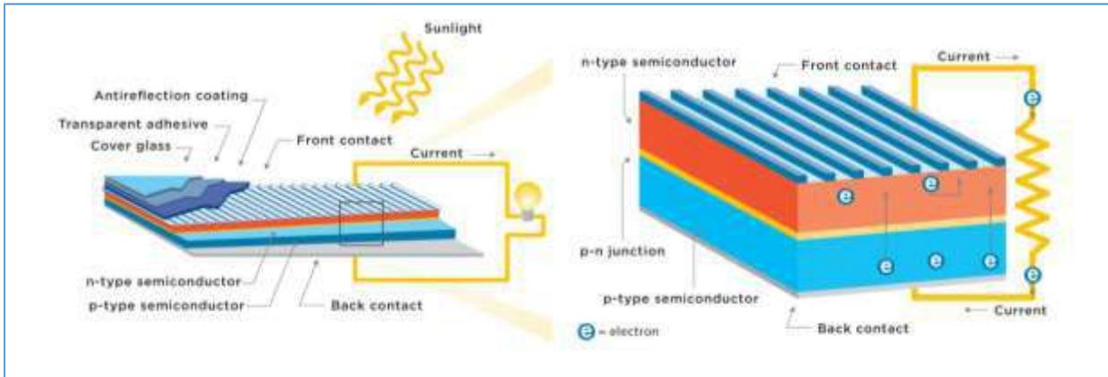
**Figure 3. Basic working of a solar cell**
