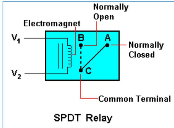
**Figure 9. Schematic of SPDT relay**
