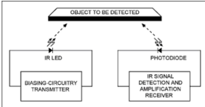
**Figure 5. Principle of IR sensor**
