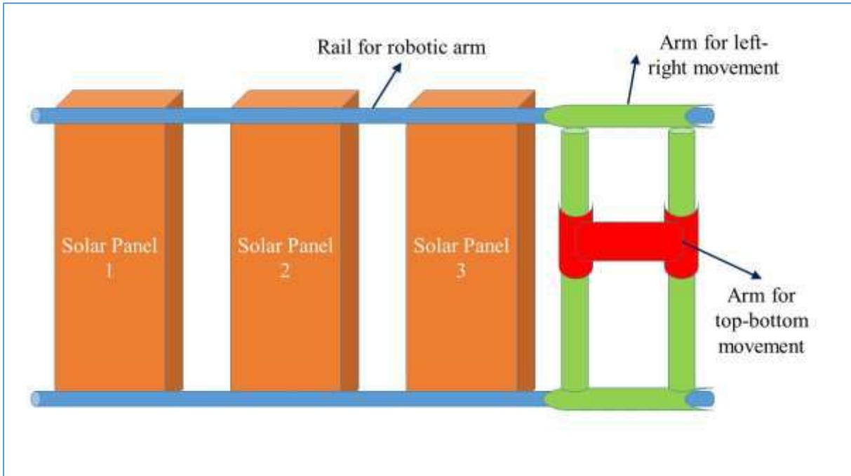
**Figure 11. Basic structure of robotic arm**
