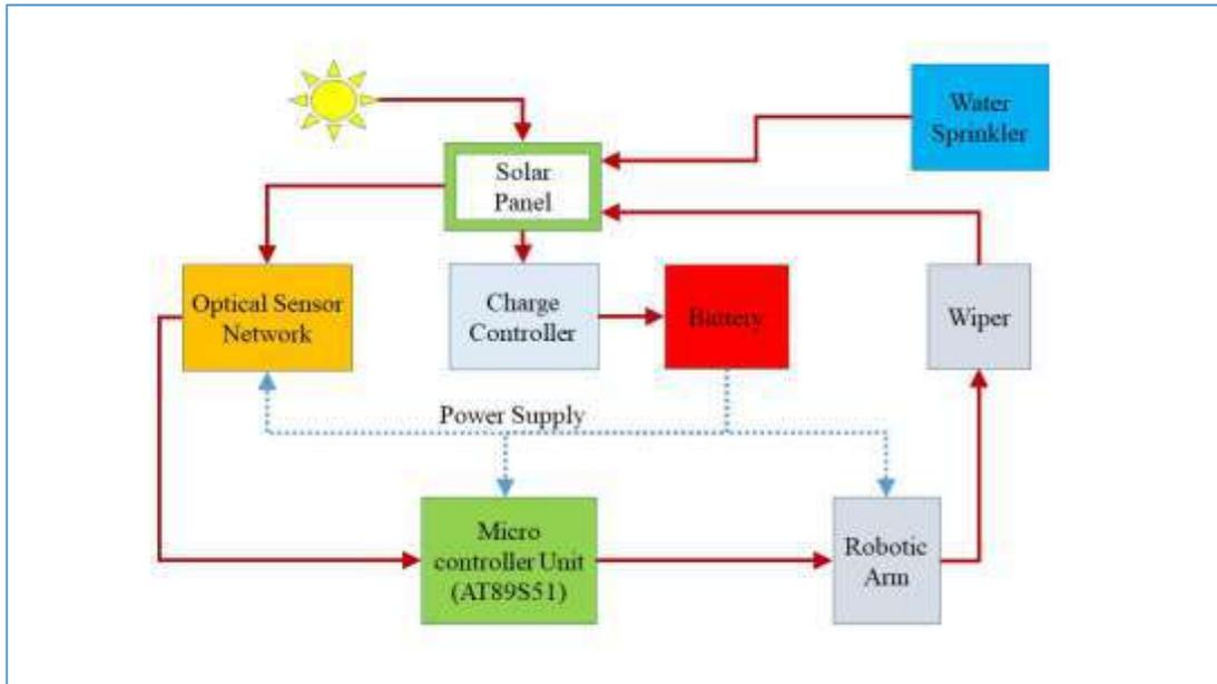
**Figure 2. Water sprinkler based solar panel cleaning system**
