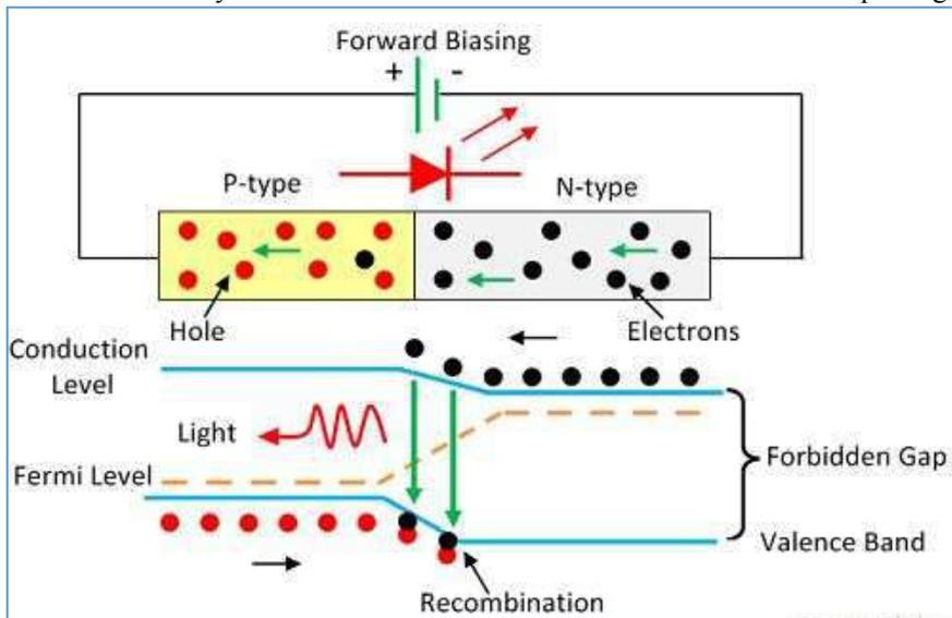
**Figure 10. Working of LED**
