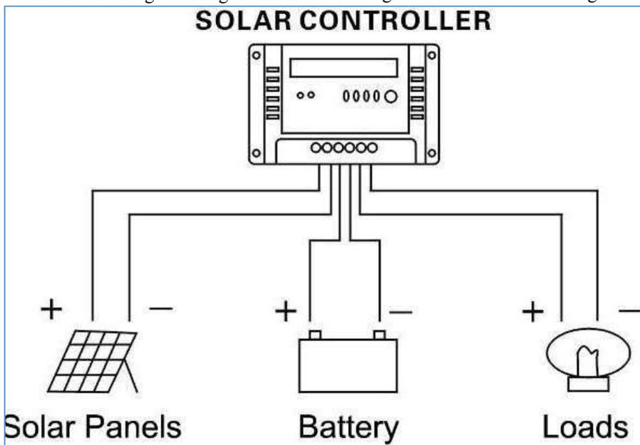
**Figure 4. Functional block diagram of charge controller**
