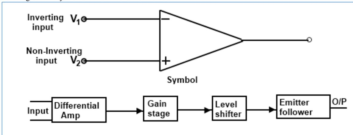
**Figure 6. Block diagram of conditioning unit**
