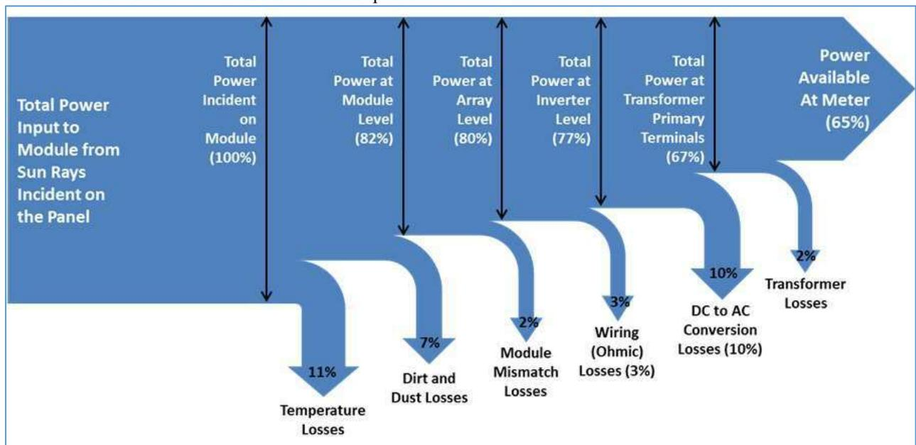
Figure 1. Electrical losses from solar energy to load
