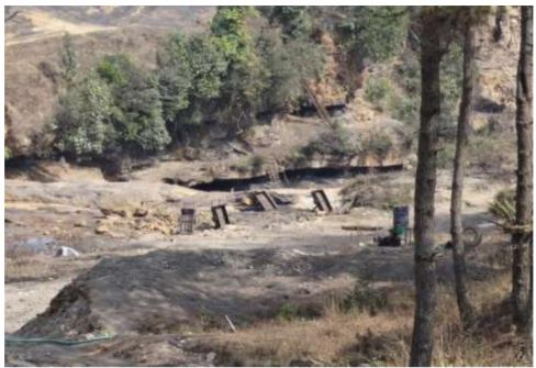
FIGURE 3. Rat holes being dug sideways into the hills of Ladrymbai quarry to reach the coal seams Source: (Field Survey April, 2017).
