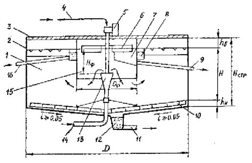
Figure-2. Flotator cooler.
