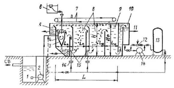
farm, water-air saturation device, pumps and other elements. [5]
