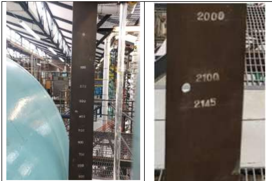
Fig. 3. The counting of the filling time of the bottom tank begins with the value of 2145 liters on the metal scale
