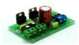
Fig.5.Power Supply Board
