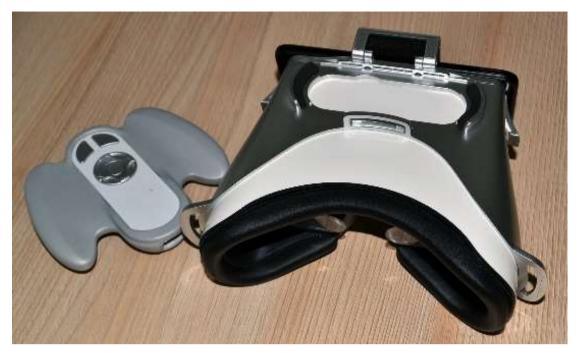
Figure 1. The composition of device for measurement the contrast sensitivity through computerized software support and the VR-glasses.
