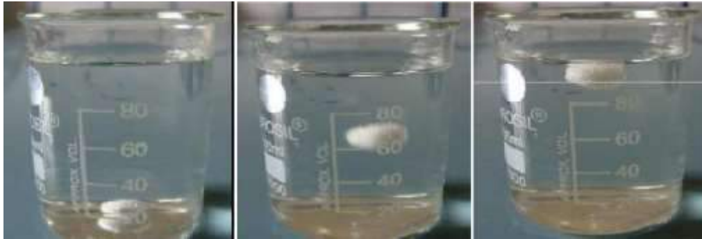
Figure 9 Buoyancy floating of formulated floating tablets
