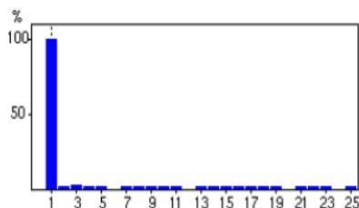
Fig 12. THD spectrum after using filter
