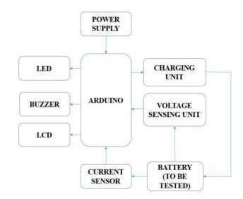
Fig.1.Block Diagram of Battery level monitoring.
