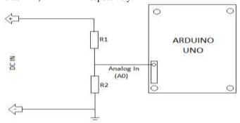
Fig. 4 Voltage divider circuit with Arduino Microcontroller.
