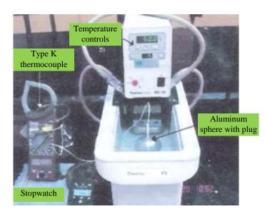
Figure 2.- Bath with aluminum sphere
