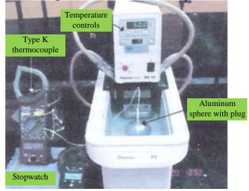
Figure 2.- Bath with aluminum sphere
