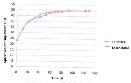
Graph 3.- Temperature profiles for aluminum sphere Theoretical temperature versus experimental temperature for aluminum sphere
