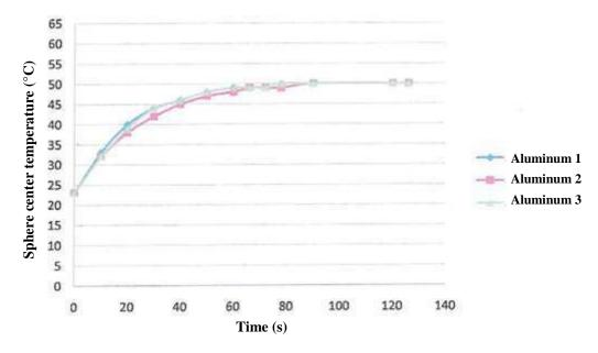
Graph 1.- Behavior of aluminum sphere Runs 1, 2 & 3 for aluminum sphere at 50°C
