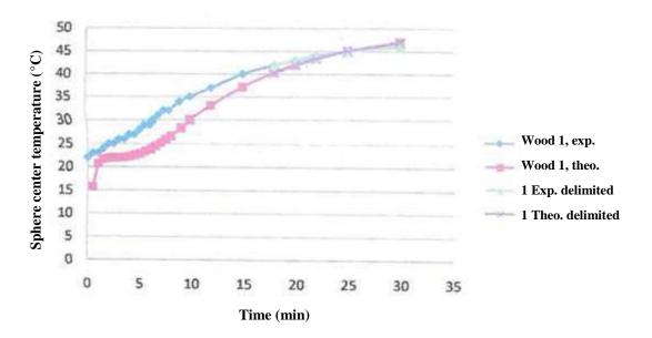
Exp. temperature vs theoretical temperature for wood
