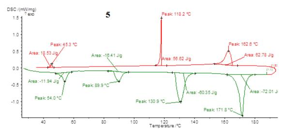
Modified transition temperatures of thermostable ammonium nitrate with dolomite additives (Photo 1)
