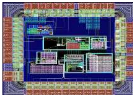
Fig. 8. Readout and 12-bit SAR ADC circuits as a front-end chip layout
