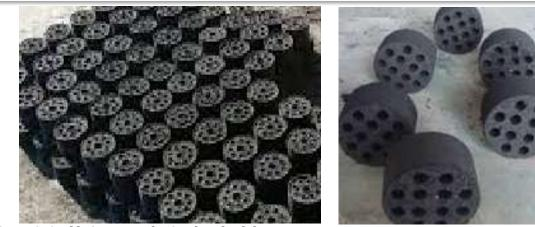
Figure 2. Coal briquettes obtained under laboratory conditions on the basis of bioorganic compounds.
