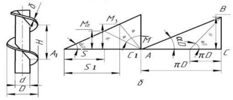
Figure 3. Scheme for determining auger performance.
