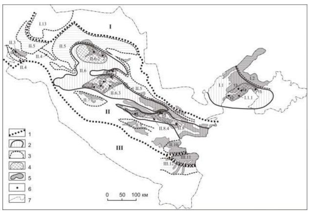
Fig. 1. - Scheme of metallogenic zoning of endogenous gold mineralization in Uzbekistan (according to Golovanov I.M., Horvat V.A., Koloskova S.M., Zavyalov G.M., Rakhmatullaev Kh.R., Dzhantuganov N.I., etc., 1997).
