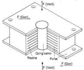
core slightly larger than the hole and using force during its installation into the hole.
