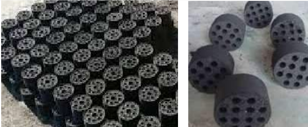
Figure 2. Coal briquettes obtained under laboratory conditions on the basis of bioorganic compounds.
