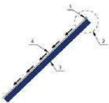
1 - perforated tube; 2 - microclimate; 3 - PVM; 4 - water film.
