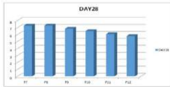
Figure 7.2.0 Flexural Strength@28day With 2% Coir Fibre
