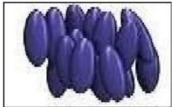
Fig. 4: Alignment in a nematic phase [5]
