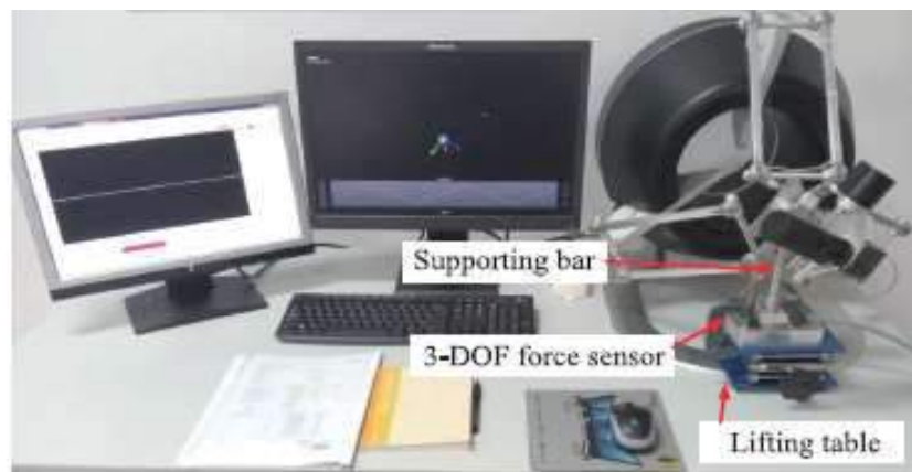
Figure 8. An experiment set up of Haptic interface between the System and the virtual environment
