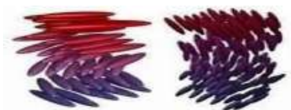
Fig. 6: Schematic of ordering in chiral liquid crystal phases [5]
