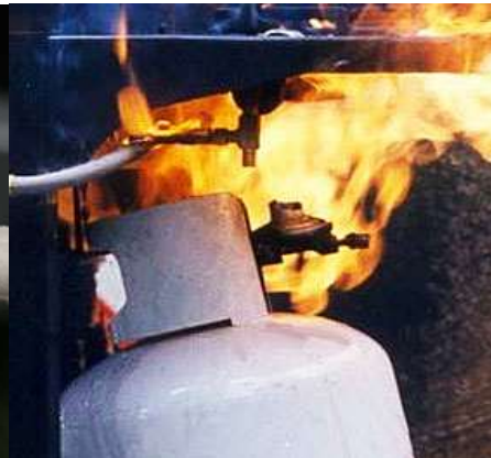
Fig 1.b LPG Leaked Contact with an Ignition Source
