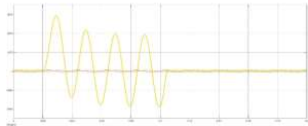
Fig 6: Line to Ground (LG) Fault Condition waveforms.
