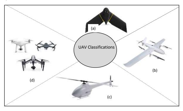
Figure 1. (a) Fixed Wing Drone (b) Fixed wing VTOL Drone (c) Single Rotor Drone (d) Multi Rotor Drone
