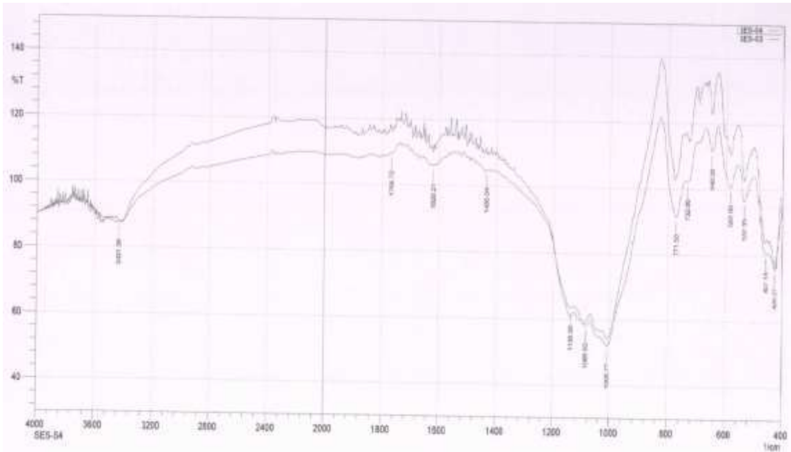
Figure-15: FTIR spectrum of concrete powder before and after adsorption of Chromium
