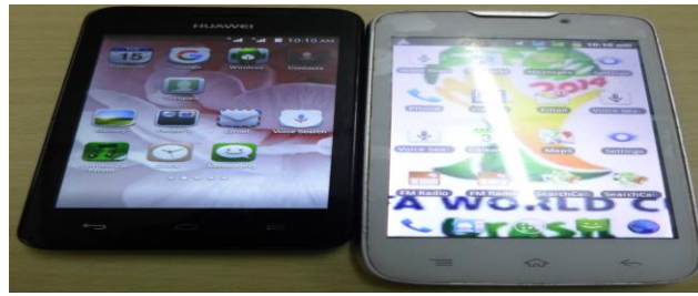
Figure 2. Placement and direction of two Mobile devices to measure RSSI data differences
