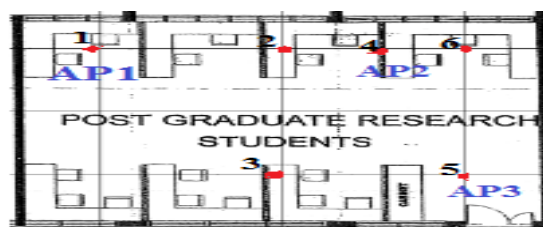
Figure 1. Location of APs and the measurement points on the Postgraduate research room
