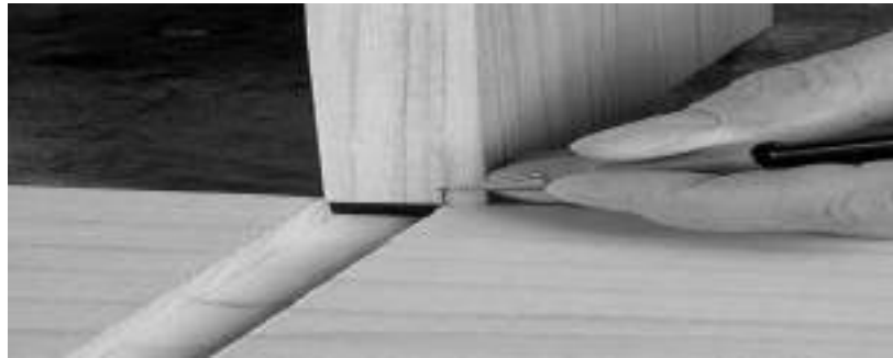
Fig 3.0 Marking out cut-off sections of the wood
