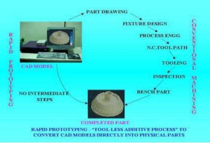
Fig.1.RP in comparison to NC machining
