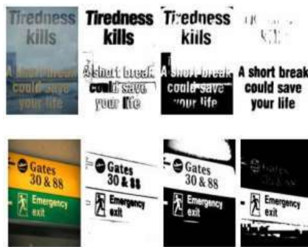
Fig.4. Multi-level binarization results of two test images
