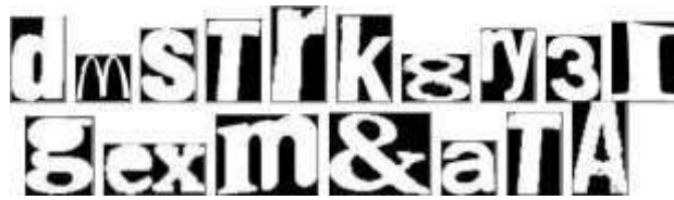
Fig.5. Samples of extracted connected components from different binarizations. Those are the most frequent type of extracted text components.
