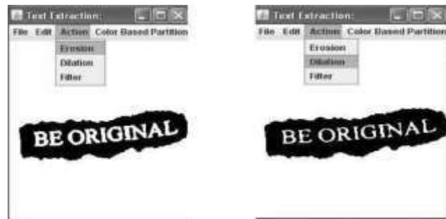
Fig.14. An example of Dilation and Erosion
