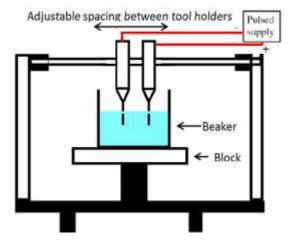
Fig. 1 ECMM Tool Fabrication Setup
