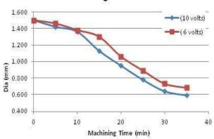
Fig 3: Variation of diameter with time Photographs of fabricated different straight micro electrodes are given in Fig.4. In some experiments, a slight taper is observed at the tip which is further reduced by increasing dipped length (L) in electrolyte.
