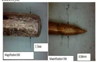
Fig. 4 Tool fabrication at 6 volt 30gm/lit NaNO<sub>3</sub> electrolyte concentration (a) Anode copper wire before machining (b) Anode copper wire after machining
