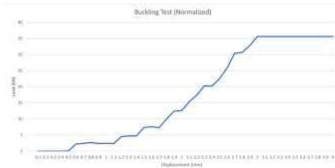
Figure 9: Load v/s displacement of normalized steel
