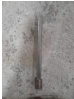
Figure 5: Specimen cap used to fix one end
