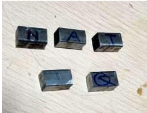
Figure 1: samples for Rockwell hardness test
