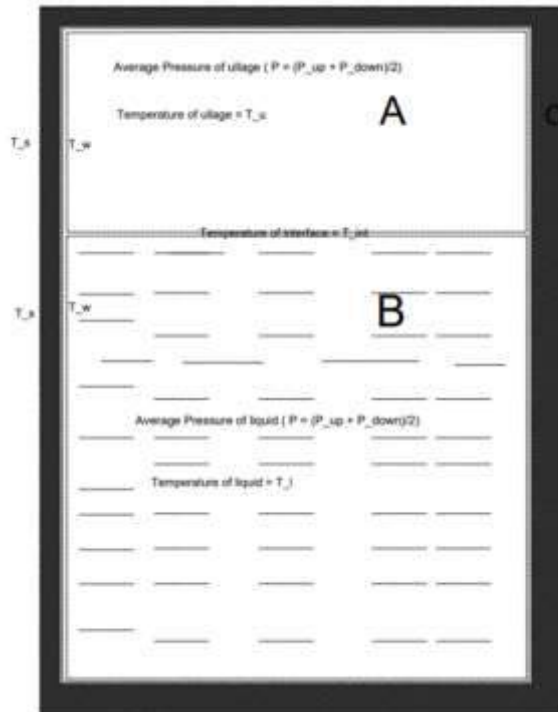
Figure 3: Distribution of nodes within the capacity of the tank and on the wall
