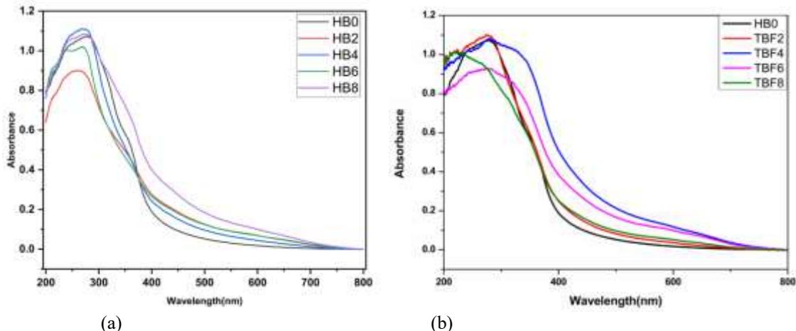
Fig 3.71 UV Spectra of untreated and treated banana fiber HPMC films
