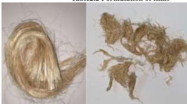
**Fig 2.1 (a) Untreated Banana Fiber (B) Treated Banana Fiber**
