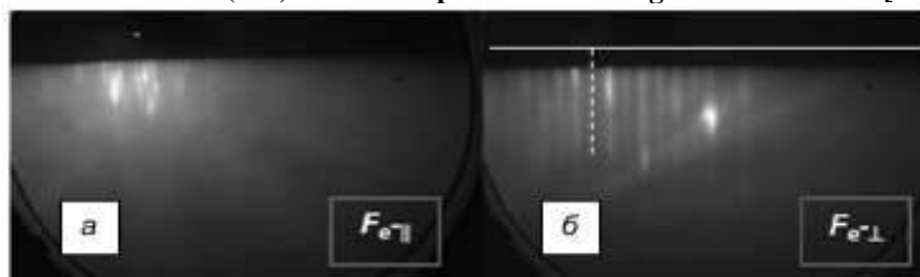
Fig. 5. RHEED pattern from a 25 nm Ga/Si(001)60 film around <011>, nucleation of the first monolayer by mixing. The surface cell (2*4) is oriented perpendicular to the edges of the terraces.[17].
