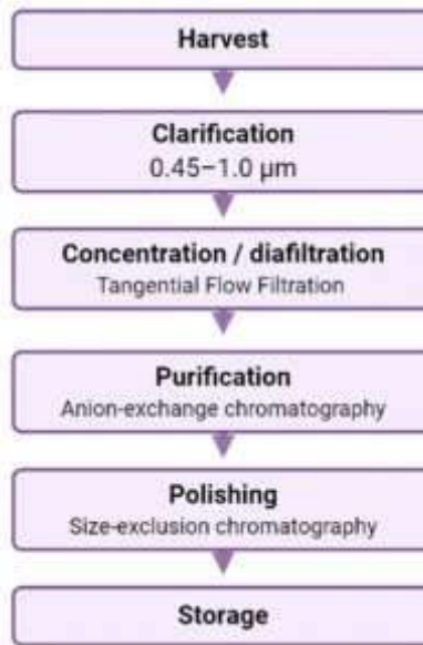
Fig 2. Flowchart for Downstream Processing of Lentiviral vectors
