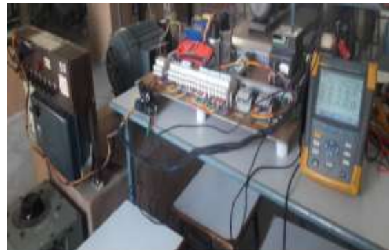
Fig 12 EXPERIMENTAL SETUP OF VFD FED INDUCTION MOTOR LOAD WITH FILTER
