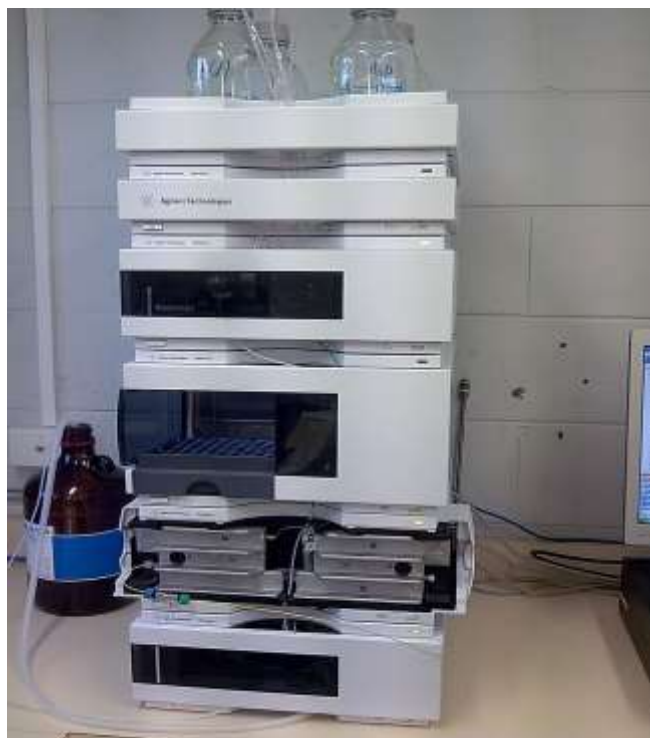
Fig:- 2. A modern self-contained HPLC.
