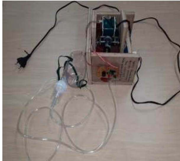
Fig-6: Compact automated Low cost portable Nebulizer
