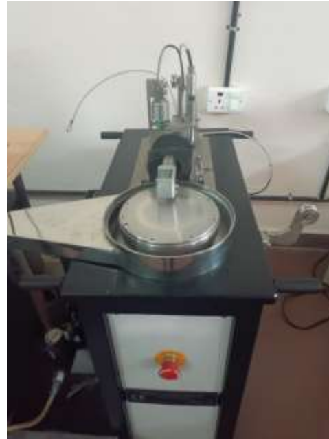
Fig 7 Pin On Disc Apparatus
