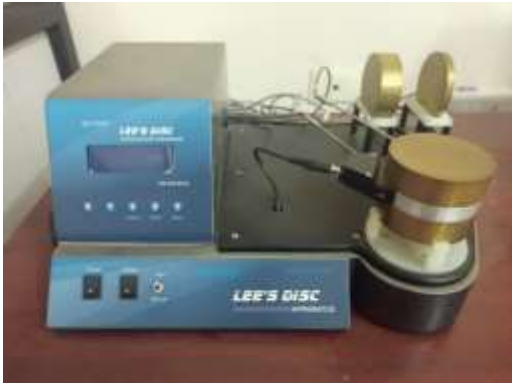
Fig 6 Lee Disc Apparatus
