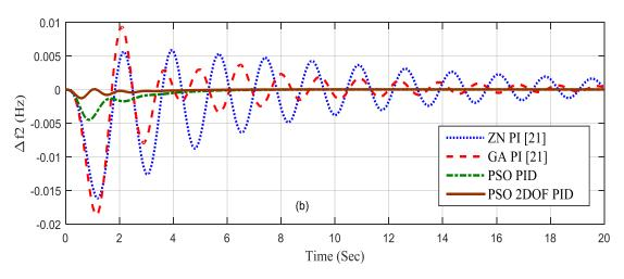
Fig1.2 Frequency deviation two area thermal and hydral system at area-2 for load disturbance of 1%
