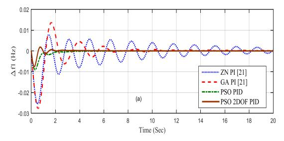
Fig 1.1 Frequency deviation two area thermal and hydral system at area-1 for load disturbance of 1%
