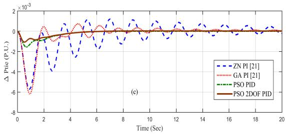
Fig 1.3 Tie line power deviation for two area thermal and hydral systems
