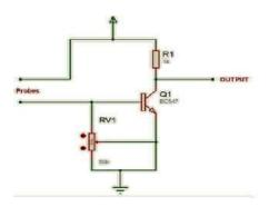
Fig.2 Circuit diagram of the Soil Moisture Sensor
