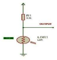
Fig. 3 Light Intensity Sensor Circuit Diagram
