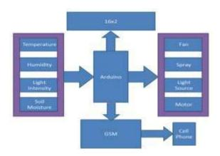
Fig. 6 Block Diagram of Proposed Remote Operating Station
