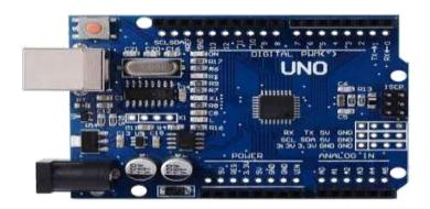
The output of the comparator is given to the digital pin 8. The Arduino is programmed in such a way that whenever there is an input high at the digital pin 8, then the TX pin i.e. pin1 gets activated and the transmitter Bluetooth module which is acting
