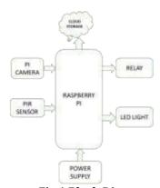
Fig.1 Block Diagram
