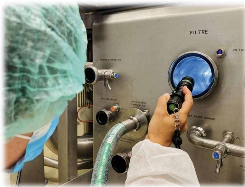
Fig.1 Visual Inspection of cleaning validation
