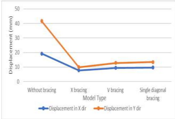
Fig 5.1: Maximum storey displacement in X, Y direction
