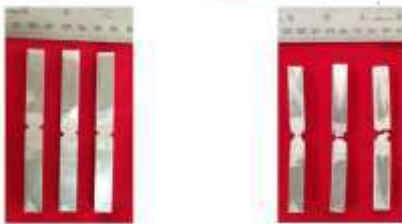
Before test After test Fig.5.6. ST+AA Welded joint notched tensile specimens
