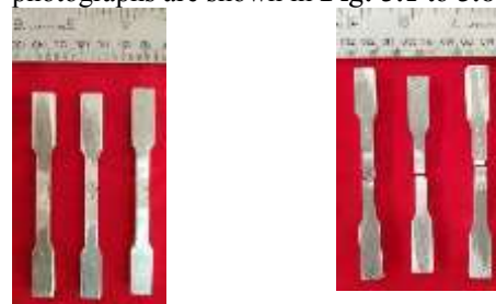
Before test After test Fig.5.1 AS Welded joint tensile smooth specimens
