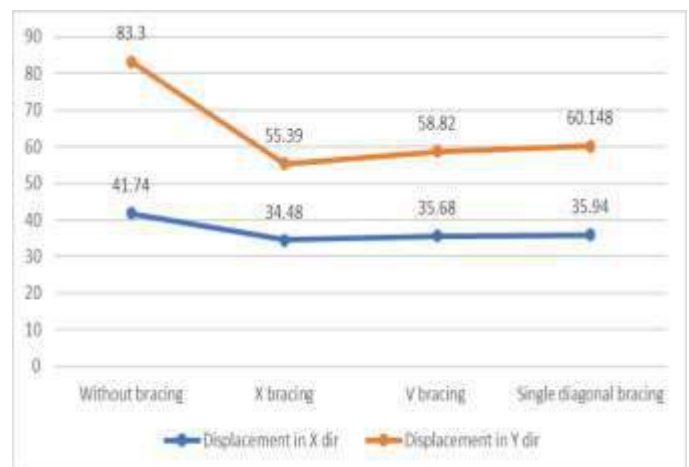
Fig 5.9: Maximum storey displacement in X, Y direction It is observed that the storey displacement in the models
