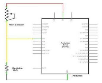
Figure 7.Schematic Diagram of Flex Sensor
