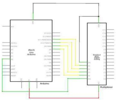
Figure 11.Schematic Diagram of Multiplexer
