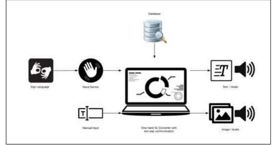
Figure 2.Digital One Hand Sign Architecture from Hearing Impaired person to Non- impaired and from Non- impaired to Impaired
