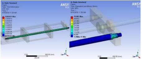
Figure 15 : Total Deformation and Von mises stress
