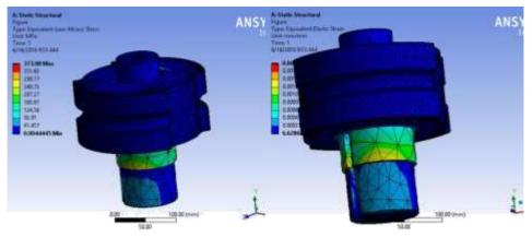
Figure 16 : Von mises stress and Maximum Principal Stress
