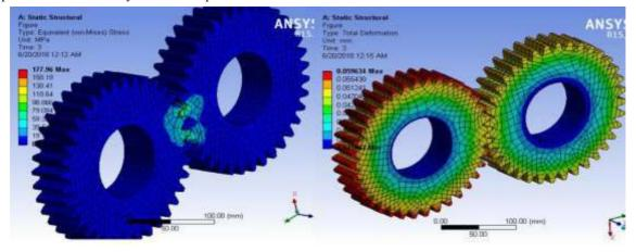
Figure 9 and represents the Von mises and the total deformation.
