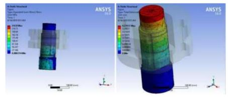
**Figure 19: Equivalent Stress and Total Deformation**
