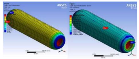
Figure 21 : Total Deformation and Equivalent elastic Strain
