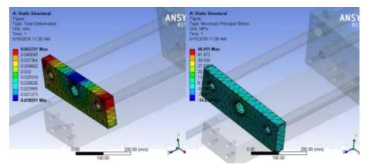
Figure 14 : Total Deformation and Maximum Principal Stress
