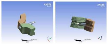
Figure 5: 3 D Model of the Roller Dies and Meshed component
