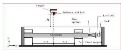
Fig2: Schematic view of test set up
