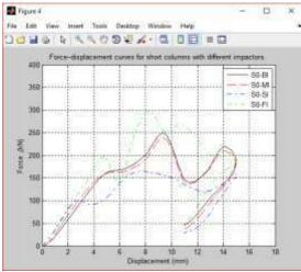
Fig6: Force-displacement curves for different indenters
