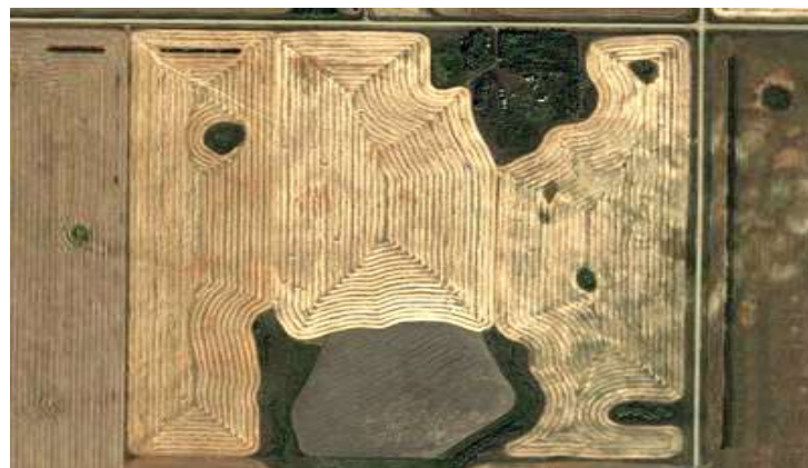
Figure 3. Space images of a field processed using satellite navigation systems.
