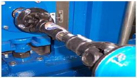
The above demonstrated drive shaft with universal joints at each end and a spline in the centre.
